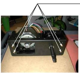
Slide the front plate off the assembly and off the shaft. Then remove the belt from the two pullys of the motor and the shaft.
