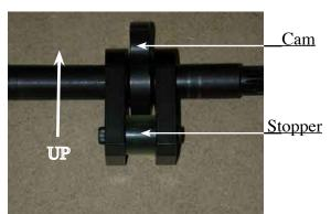
Be sure to center the shaft with the cam in the upwards position and the Stopper dangling downwards.
