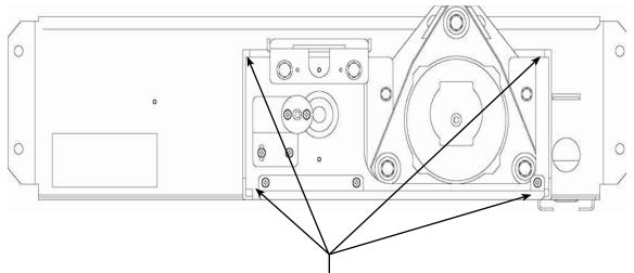
Remove the Hardware from the control panel plate and separate the Steering Handle Assy from the plate.
