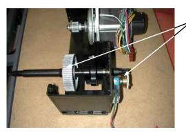
Slide the shaft out of the housing having a care for the volume pot in the rear. Using a 2mm Allen wrench, remove the pully from the shaft.
