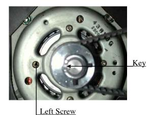
Then turn the motor until the key points to the left screw on the motor.
