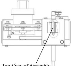
Top View of Assembly Screws are beneeth this plate.
